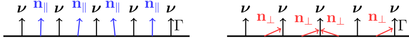
Figure 2.1. Left: Illustration of homeotropic anchoring. Here the director \mathbf{n} , which we denote by \mathbf{n}_{\parallel} , is closely aligned with the outward normal vector \boldsymbol{\nu} ; the closeness of alignment is controlled by the constant w_0 . Right: Illustration of planar degenerate anchoring. Here the director \mathbf{n} , which we denote by \mathbf{n}_{\perp} , is closely aligned tangent to the surface; the closeness of alignment is controlled by the constants w_1 and w_2 .
